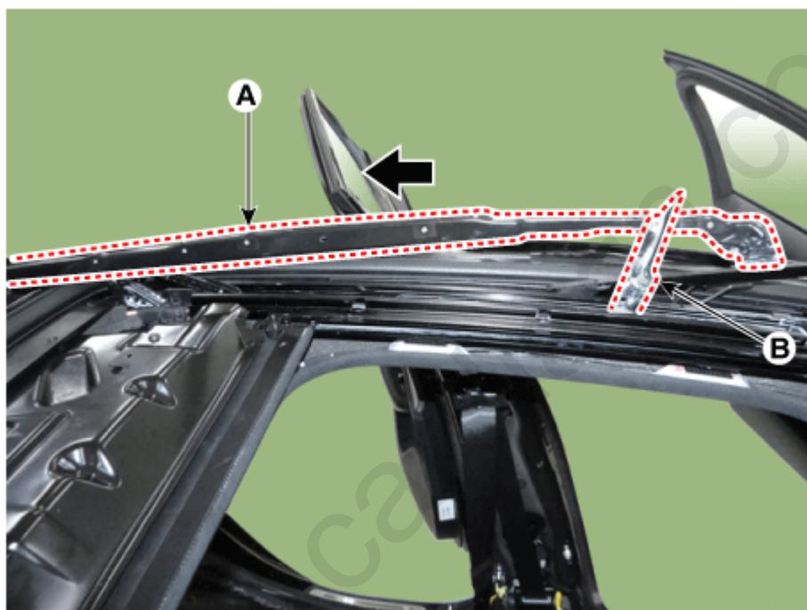
7. Remove the front slide shoe(A) by pushing direction of an arrow from mechanism guide.
