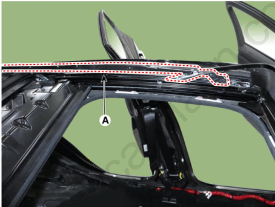
3. Remove mechanism rail front locator after loosening the mounting screw.
